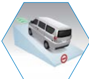
HSA (Hill Start Assist) Prevents rollback(2 sec.) on slopes by holding the brakes
